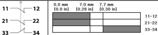
**Switch Code 30 – 3 NC****Schaltercode 30 – 3 NC****Code d'interrupteur 30 – 3 NC****Codice interruttore30 - 3 NC****开关代码30 - 3NC****스위치 코드 30 – 3 NC**
