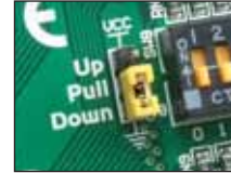
Figure 21-2: J2 in pull-down position
