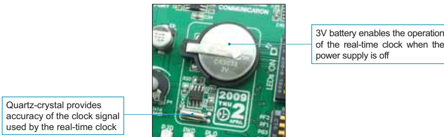
Figure 14-1: Real-time clock
