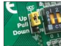
Figure 21-3: J2 in pull-up position
