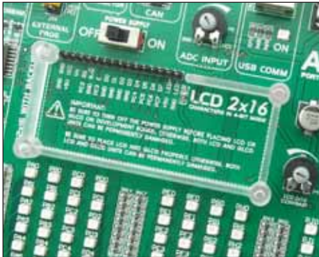
Figure 18-1: Alphanumeric LCD display connector
