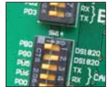
Figure 13-4: DS1820 is connected to the microcontroller via the PG0 pin
