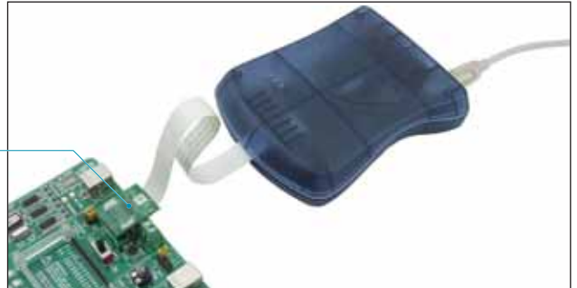
Figure 5-2: JTAGICE mkII connected to the board
