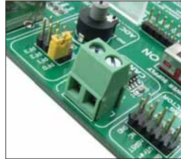
Figure 11-2: CAN module connector
