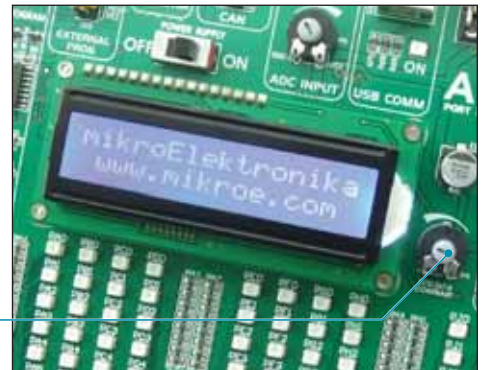
Figure 18-2: Alphanumeric 2x16 LCD display
