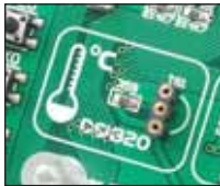
Figure 13-1: DS1820 connector (DS1820 is not placed)
