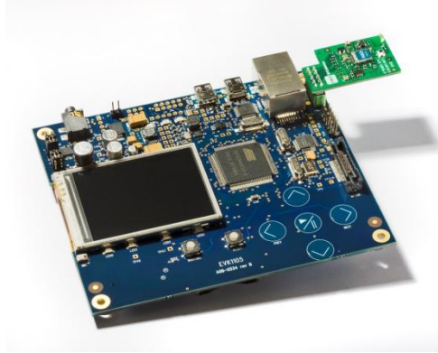
* Photo of the SPB105 connected with the SPI-card interface on the EVK1105. Ready-made downloadable reference designs can be started within minutes and development can start at once.
