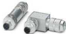
Bus system connectors for assembly with Pg9 screw connection, crimp connection, IP67, 5 – 8 mm cable diameter, for Ethernet and PROFINET
