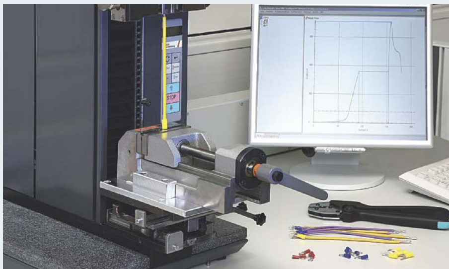
Conductor pull-out test
